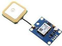
**Fig.5 NEO-6M GPS Module**
