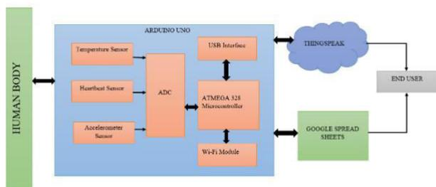
Fig.10 Schematic Diagram Of Implementation Model
