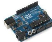
Fig. 3 Arduino Uno with Atmega 328
